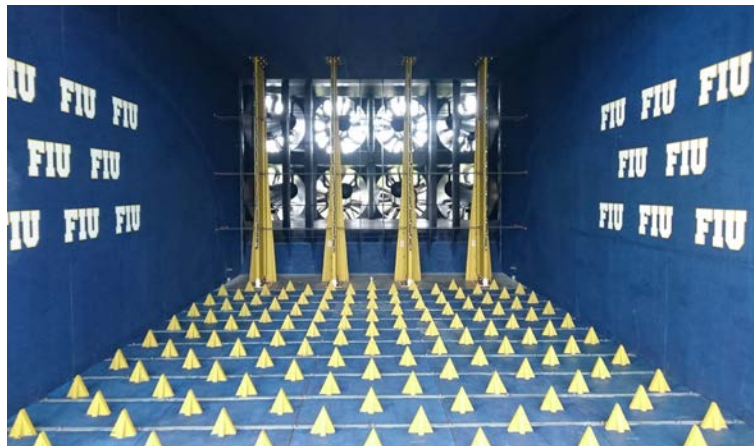
Figure 4-2. The WOW flow chamber with four spires and floor roughness elements
